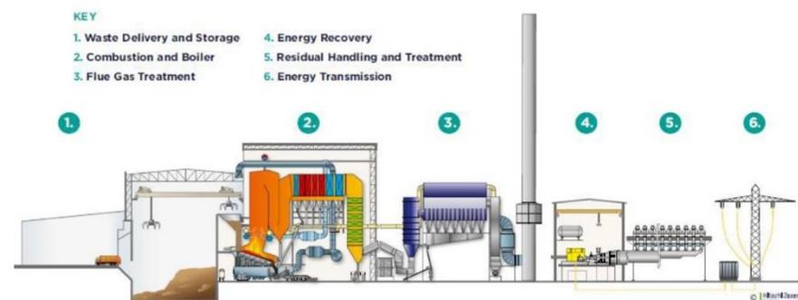
**Figure 2 Diagram of the Process Flow Through an Energy Recovery Facility**
