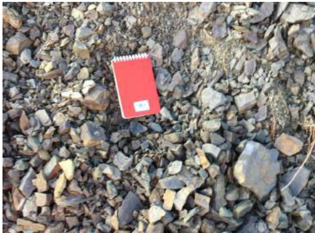
Photograph 6: Spalled material present at base of western excavation, naturally forming blocks of approximately 50-130mm in size.
